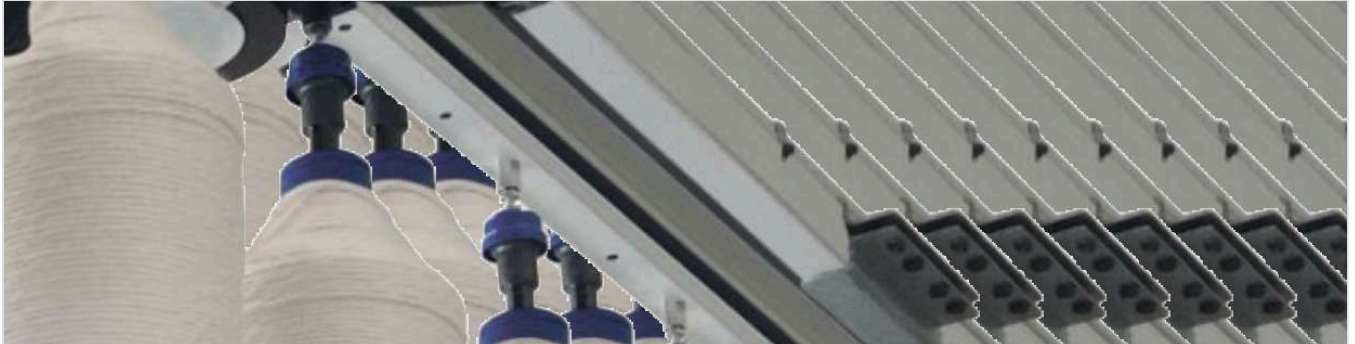
IBTS — OVERHEAD ROVING BOBBIN DELIVERY AT THE RING FRAME CREEL
